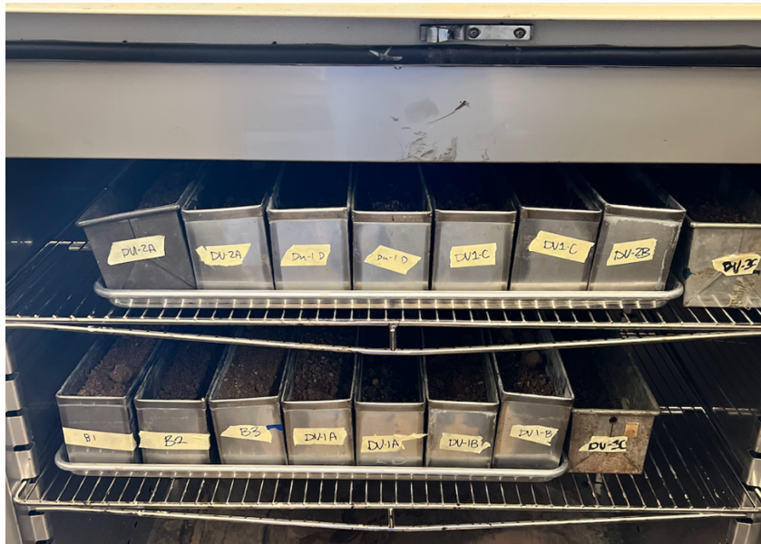
Figure 4.1: Samples Drying in the Oven
